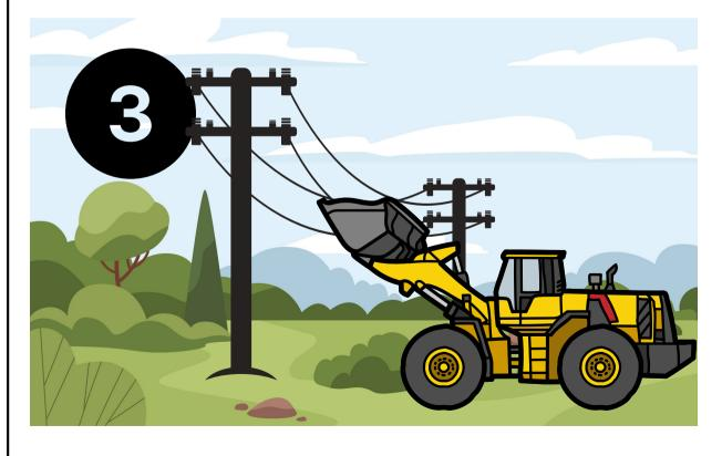
The machine has its front loader up and the driver is not aware of the power cables above.
